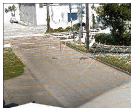
Generation of cross sections with generate planes, to check for verticality
