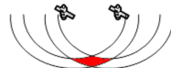
Poorly spaced satellites – high uncertainty of position
